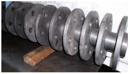
Typical agitator assembly with 10" diameter disks and 3" diameter spacers
