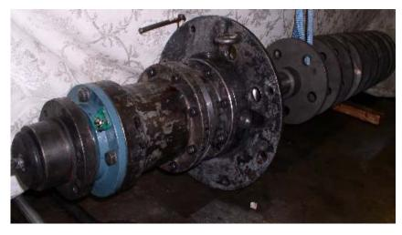
Agitator assembly being overhauled at the factory
