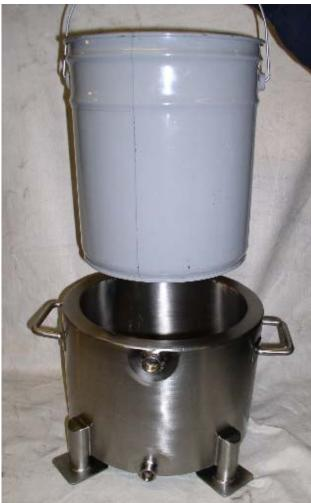
PAIL/KETTLE, CHILLER, STANDARD 5 GALLON PAIL INSERT, HEATING/COOLING/CHILLING, FLAT BOTTOM, INTERNAL SHELL SLIGHTLY SLOPED, SHELL JACKET, 75 PSIG, MAX.
