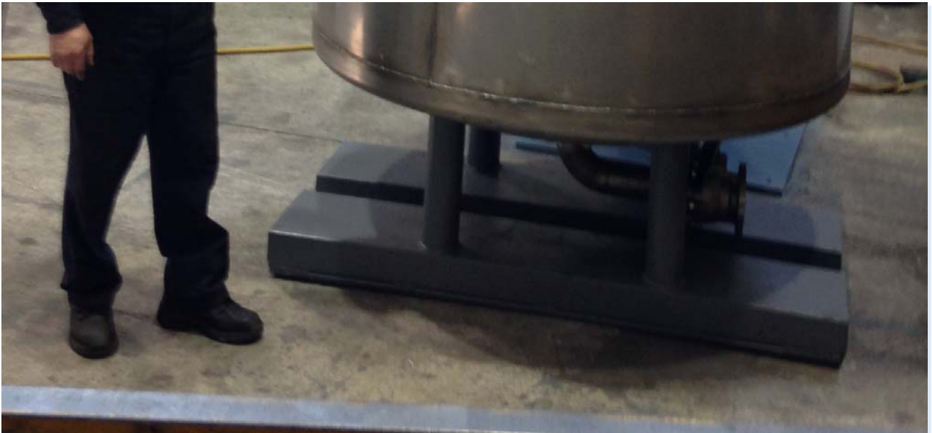
Drain Assembly: 3" flanges, 3" pipe, 3" ball valve for 600 gallon tank, all SS304
