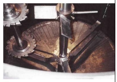
10 HP variable high speed disperser 600 to 1800 rpm (2) hsf-08 high shear blades
