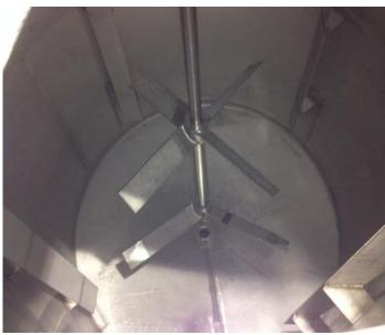
SERIES 3021 MIXER, BLENDER, AGITATOR, FIXED LOW SPEED, MOUNTED ON MIXING TANK, MIXER, MODEL FSB-150-84-EX/SS TANK, MODEL TFD-2250-84/96-SS
