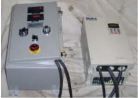
The Vector Drive Controller in NEMA 1 enclosure is shown on the right. The Remote Control Box in NEMA 12 enclosure is shown on the left (as you look at).
