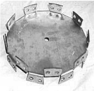
The HSO style blade offers high pumping action and high shear. The hole pattern allows for maximum shear generation with less horsepower. Other process characteristics are similar to the HSF style blades.
