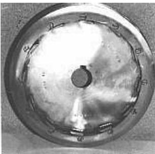
The HSD style blade is characterized as the Ring/Disk blade and offers all the advantage of a rotor/stator assembly while retaining the versatility of a single blade design. The inside sharp teeth shear pigments agglomerates and discharge materials at great speed and pressure through the slots and against the surfaces of the deflected rings. Mixing materials are quickly reduced in size with little heat accumulation.
