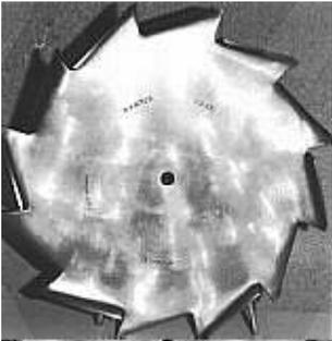
The HSG style, high vane blade, generates a high pumping action which tends to mix the entire batch efficiently, resulting in high speed blending with low shear, but with excellent flow and circulation. It is used in heavy bodied mixes that require higher shear as obtained from paddle agitation.
