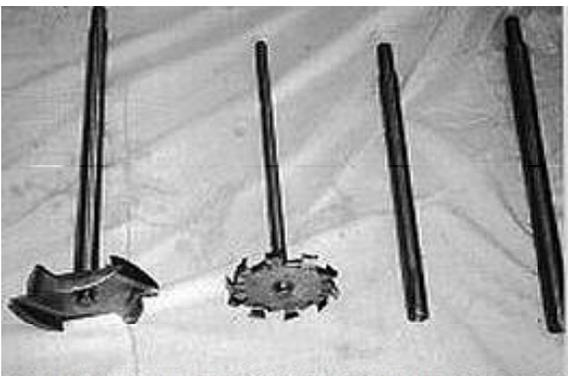
Shafts for Mini Impellers in SS304.
