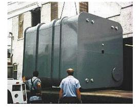
Square Tank, vertical, with sloping bottom, back to front and from sides to middle, on legs or flat slab mounted, top manhole, top & side fittings. Top 1/3 section bolted with gasket for low door building entry.
