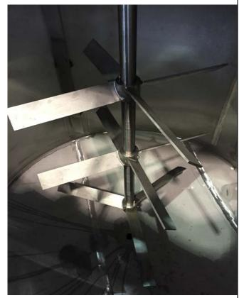
SERIES 3021 MIXER, BLENDER, AGITATOR, FIXED LOW SPEED, MOUNTED ON MIXING TANK
