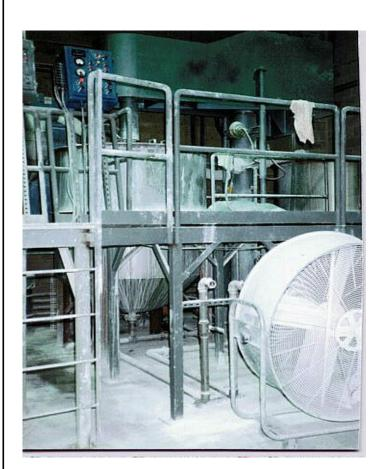
The top picture shows a Dantco post mounted, variable speed, Disperser, Series 2030, 100 HP, explosion proof, with (2) SS304 tanks with tapered bottom, mezzanine mounted, with hinged tank covers, fill piping and flow meters, drain piping hooked-up to diaphragm pumps, control panel with push button controls, digital tachometers and ammeters. Visible also is the working platform built by the customer. This heavy duty Disperser system is used to process latex paint.
