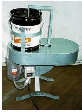
SERIES 3001 MODEL DPM-075-46-EX 5 GALLON PAIL MIXER FIXED LOW SPEED (46 RPM) PORTABLE
