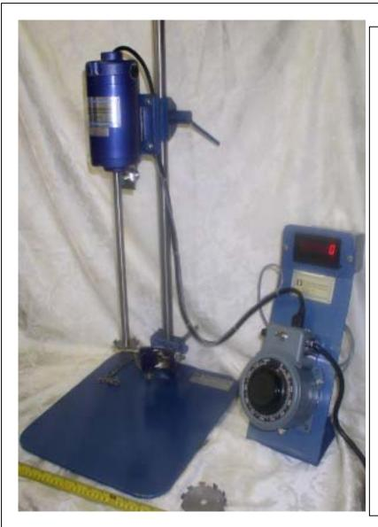
**SERIES 503B** LABORATORY DISPERSER VARIABLE HIGH SPEED AC MOTOR, OPEN
